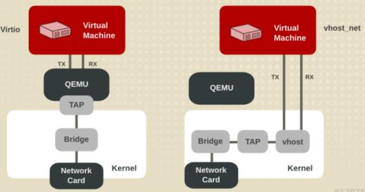
https://access.redhat.com: "vhost\_net moves part of the Virtio driver from the user space into the kernel. This reduces copy operations, lowers latency and CPU usage."
